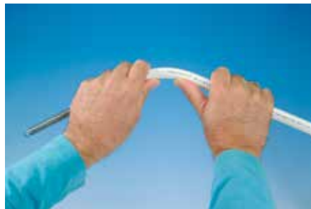
Bending with an internal bending spring
