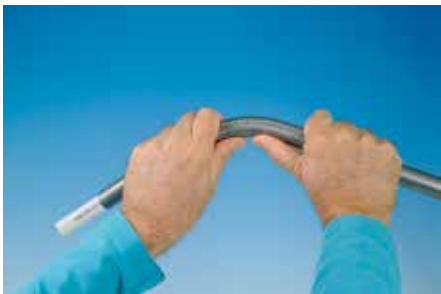
Bending with an external bending spring
