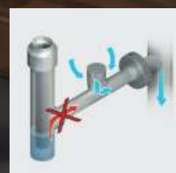
Version with venting valve "AIRPIPE"
