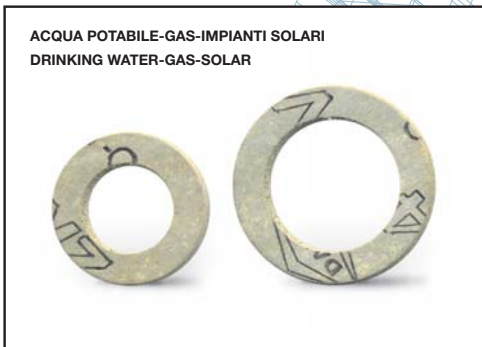
GUARNIZIONI AFM34 APPROVATE. FIBRA ARAMIDICA TEMPERATURA: FLUIDI 250°C VAPORE MAX 200°C AFM34 GASKETS APPROVED. ARAMIDE FIBRES. TEMPERATURE: FLUIDS 250°C STEAM MAX 200°C
